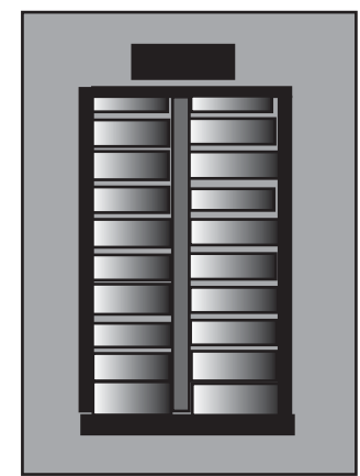
This One Uses Circuit Breakers
